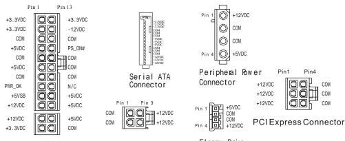
Main Power Connector +12V Power Connector Floppy Drive Power Connector
