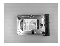
3. Align 3.5" HDD hinges to the rail and slide it slowly into the metal frame.
